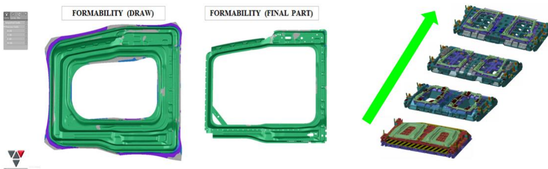
Fig. 3: Left, formability output of draw and final part form. Right, die-set design.
