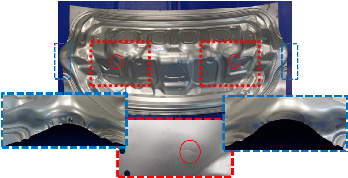
Figure 2. Impression of the trunk lid inner part after the forming operation with critical regions showing splits or critical thinning (red) and wrinkles (blue)
